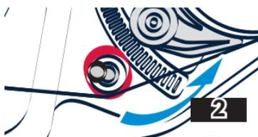
To adjust visor friction, tighten (Fig. A.) or loosen (Fig. B.) the adjustment screw using the Allen key provided here. Caution: adjust in several steps without forcing, to maintain equal pressure on both sides.
